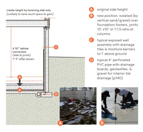
\$2,500-\$4,000 demolition of existing structures + slab \$2,000-\$3,000 basic slab pour
