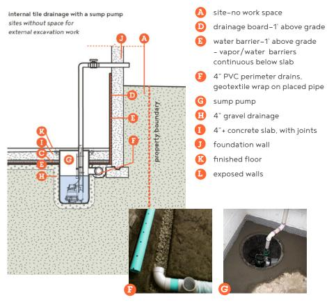
\$3,500-\$6,000 drainage plane, insulation for slab \$6,000-\$10,000 sump pump & tile installation
