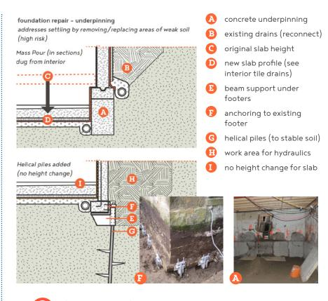
\$20,000-\$40,000 concrete is less, helical piles more Underpinning should only be done if absolutely necessary to prevent structural failure. Digging beneath your foundation has the potential to destabilize your entire house and should be done in small sections, with extensive supplemental support. It may void your home insurance so discuss extensively with your engineer before pursuing underpinning.
