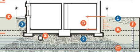
\* lots with tight offsets have limited areas to excavate or alter soils to address drainage or lateral soil loads
